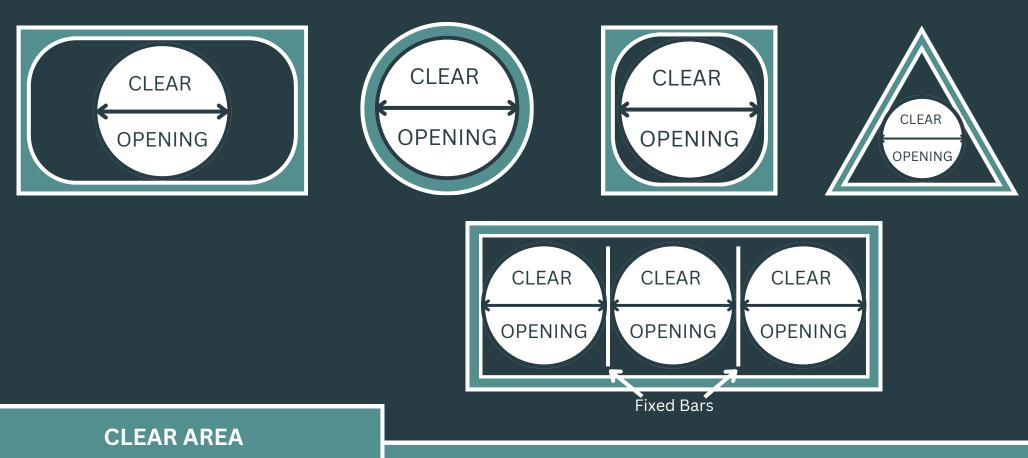
Defined by international standards, the term 'Clear Area' pertains to the unobstructed space within the seating of a manhole cover's frame, as clearly depicted in these diagrams. It's important to note that this differs from the overall size, which encompasses the external dimensions of the frame.
